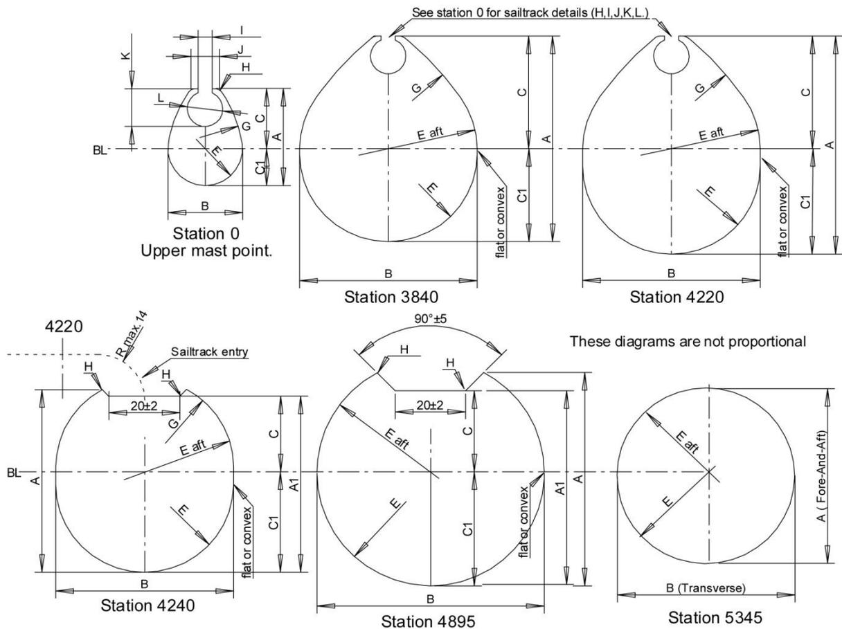
**BOOM MEASUREMENT DIAGRAM**
