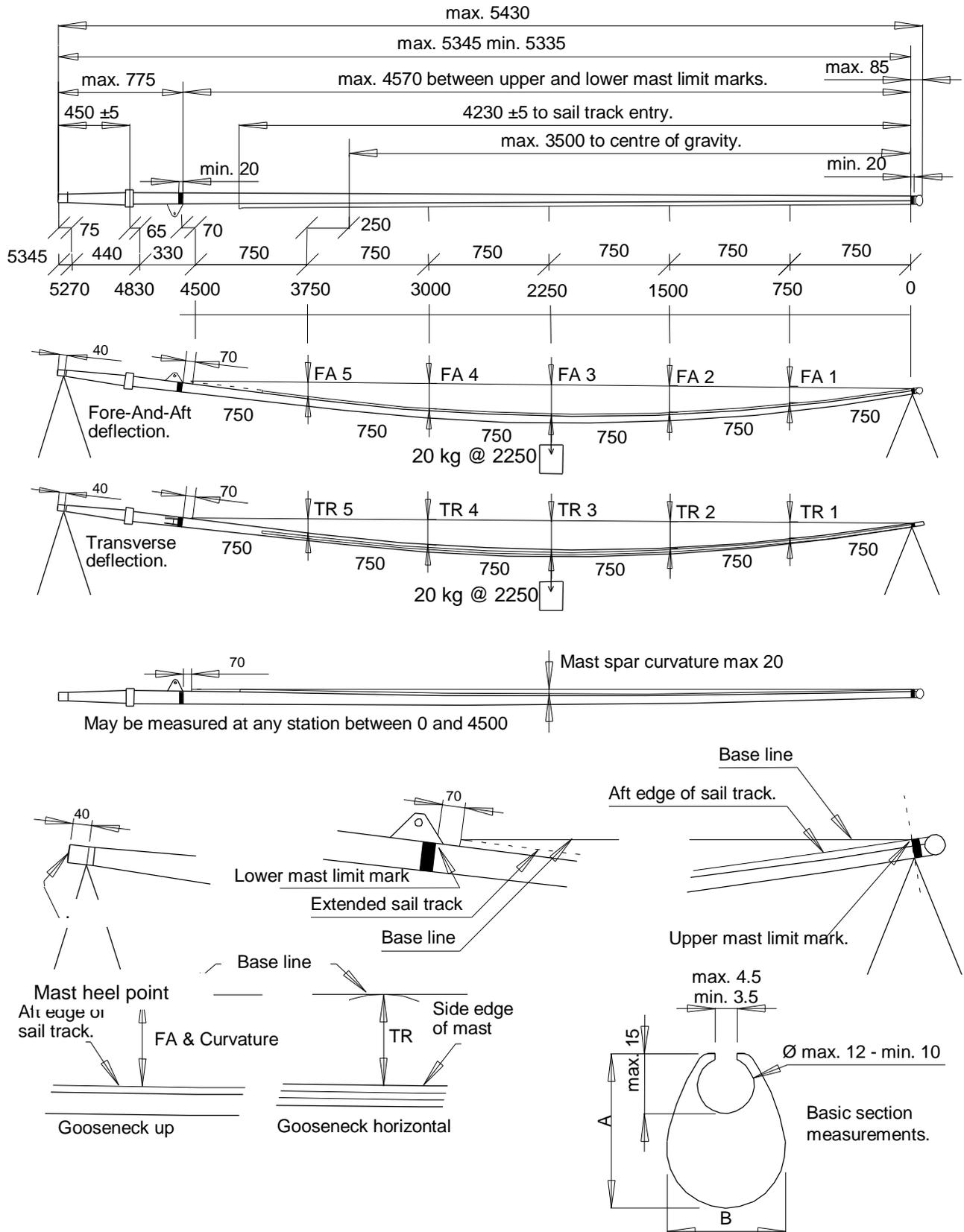
**MAST MEASUREMENT DIAGRAM SHEET 2 OF 2.**
