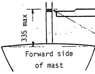
The upper edge of forward end of the boom shall not be lower than the top of the lower band on the mast.
