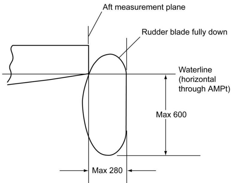
**RUDDER FITTINGS MEASUREMENT DIAGRAM**
