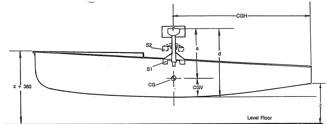
A 90 degree knife edge for the support beam pivot axis is recommended
