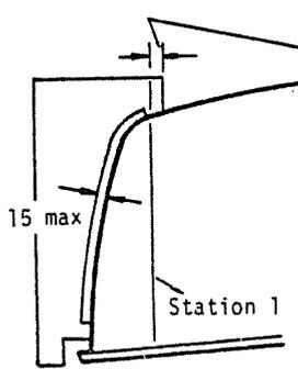
The stem template shall be set with its 'nibs' touching the hull and with its aft edge forward or aft of station 1 by a distance equal to the difference in hull length from the mean length (3350mm) taking account of sign (i.e. + or -).
