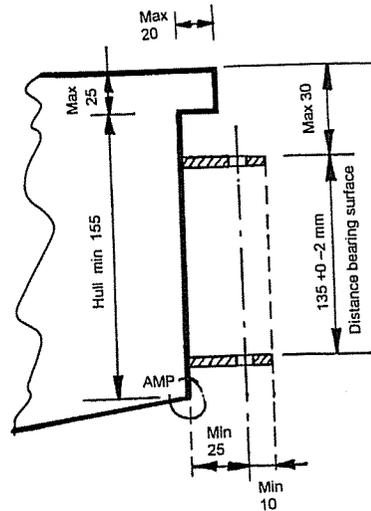
Diameter of holes in the bearing Surfaces min 8.0mm
