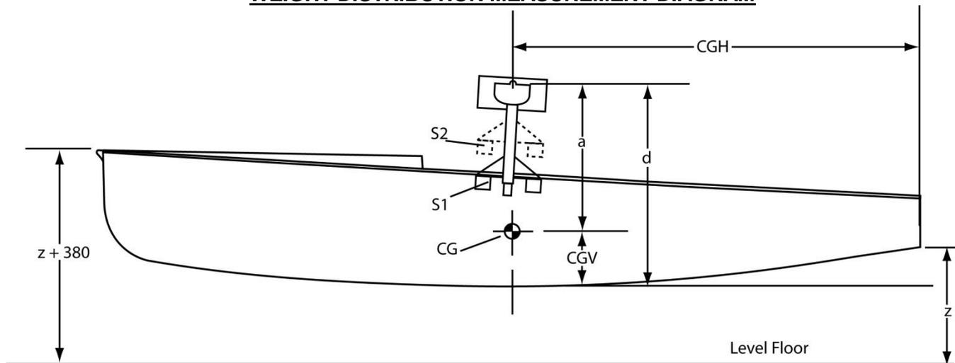
A 90 degree knife edge for support beam pivot axis is recommended
