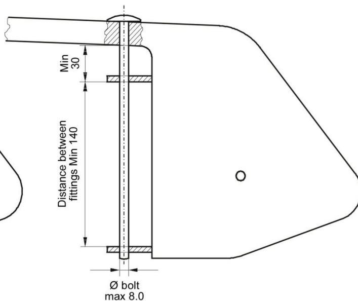
**MAST MEASUREMENT DIAGRAM SHEET 1 OF 2.**
