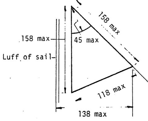
The headboard shall be incised in the triangle. The top of the headboard shall not lie more than 45mm below the top of the triangle. The base shall lie on the 118mm line totally or partially. No part of the headboard shall be more than 138mm from the luff of the sail including the bolt rope.
